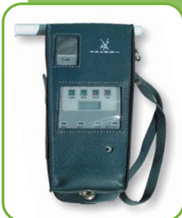
Left: Police breathalyser device for detecting alcohol on a driver's breath
