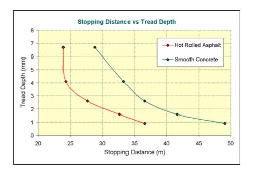
From the graph of results, it can be seen that the stopping distances start to increase dramatically at tread depths of below 3mm.
