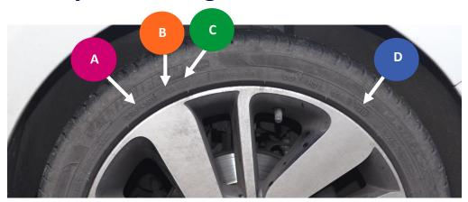
A shows the **tyre size**. The code shows the tyre's width (205mm), height (45% of the width) and rim diameter (17 inches). Radial tyres are marked with R. Almost every new tyre manufactured now is a radial tyre.
