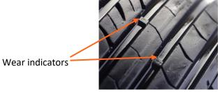
2. 20p test – take a 20 pence coin and insert it into the tread grooves of the tyre. If you can see the outer band on the coin, your tyres are likely to be above the legal limit. However, if the outer band is visible, your tyre could be below the legal limit If this is the case, take your vehicle to a professional for checks, as the tyre could need to be replaced <sup>2</sup>.
