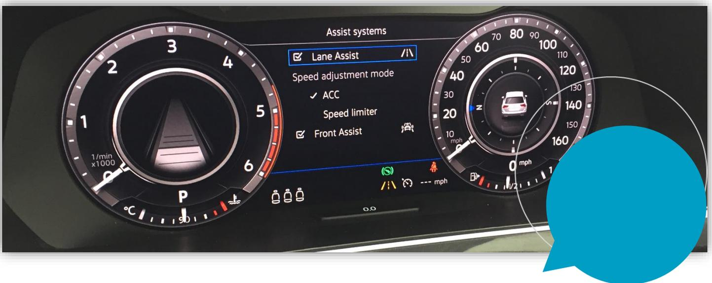
Drivers must not rely on such systems to take control of the vehicle for them. If lane markings are faded, inconsistent, or the windscreen is not clean the system may not intervene as expected. These systems generally deactivate if they detect that the driver is not holding the steering wheel. Driver fatigue can occur at any time of the day or night so adequate breaks from the wheel should always be planned in to a journey.
