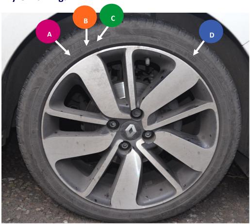
A shows the **tyre size**. The code shows the tyre's width (205mm), height (45% of the width) and rim diameter (17 inches).
