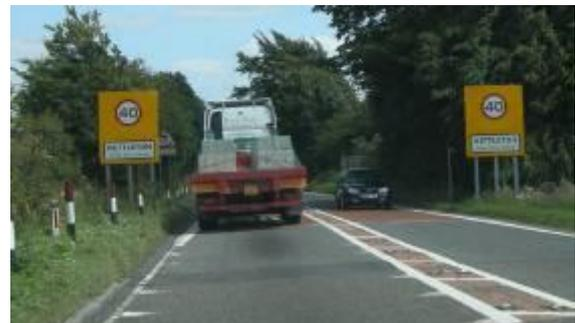
Figure 5: Transition with coloured road surface
