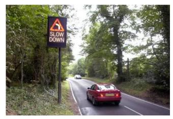
Figure 6: Vehicle activated curve/bend warning sign (driving on the left)
