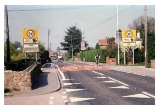
Figure 3: Gateways at a speed limit transition
