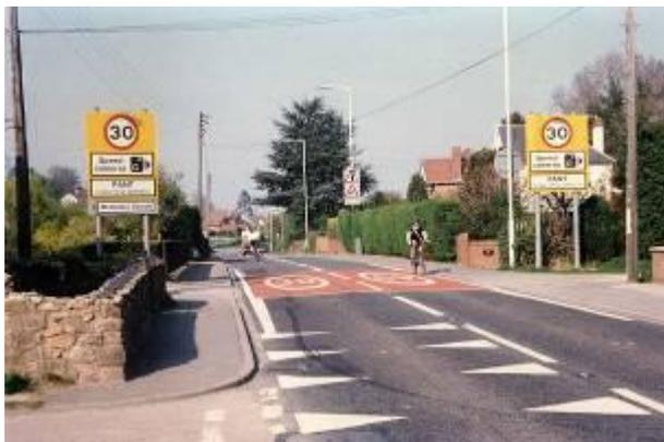
Figure 3: Gateways at a speed limit transition
