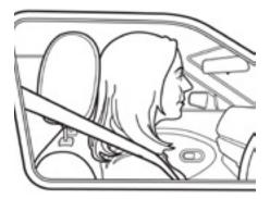
The head restraint should be as close to the rear of the head as possible.
