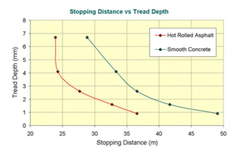
From the graph of results, it can be seen that the stopping distances in the wet start to increase dramatically at tread depths of below 3mm. At the legal minimum tread depth of 1.6mm, the stopping distance increased by 36.8% on the hot rolled asphalt and 44.6% on the smooth concrete
