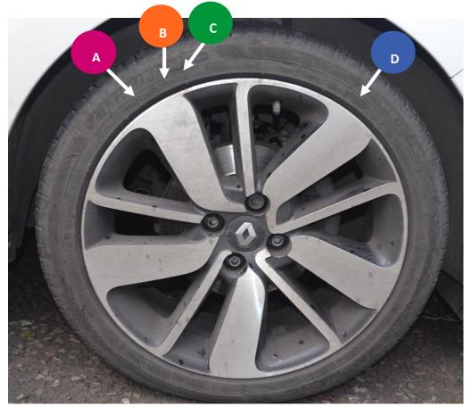
A shows the **tyre size**. The code shows the tyre's width (205mm), height (45% of the width) and rim diameter (17 inches).
